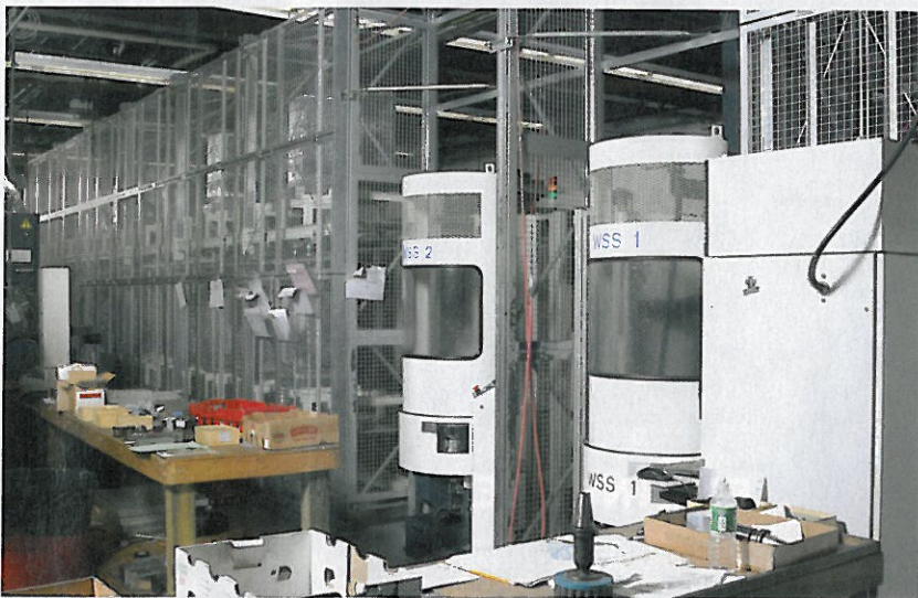
Sandy Bay's MMC2 contains two worksetting stations with 24 pallets feeding three Makino a51 HMCs, providing the flexibility to run many jobs at once without major operator intervention.
